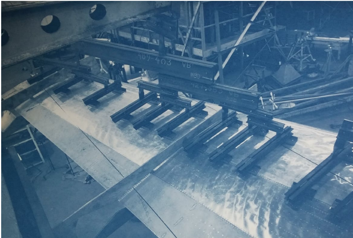
US Navy R4D (DC-3) Wing Proof Test – Extent of Buckling at 80% of Limit Load
