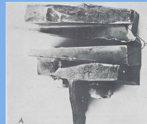
Wing Joint at WS187 Failure – Spar Cap and Fitting are 75ST Material
